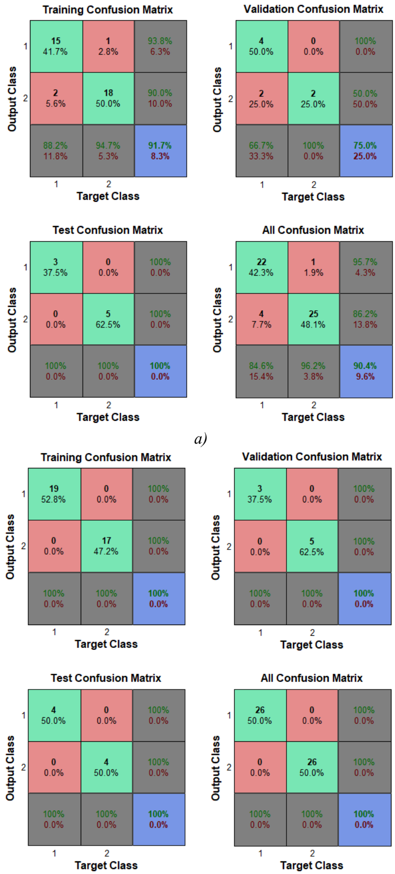
Fig. 3.11. Classification matrices for the synthesized FFNNs for quantitative identification of operating tensorresistive transducers for a) one and b) two input variables
